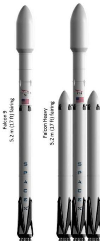
**Figure 4-2 SpaceX Falcon 9 and Falcon Heavy [1]**
