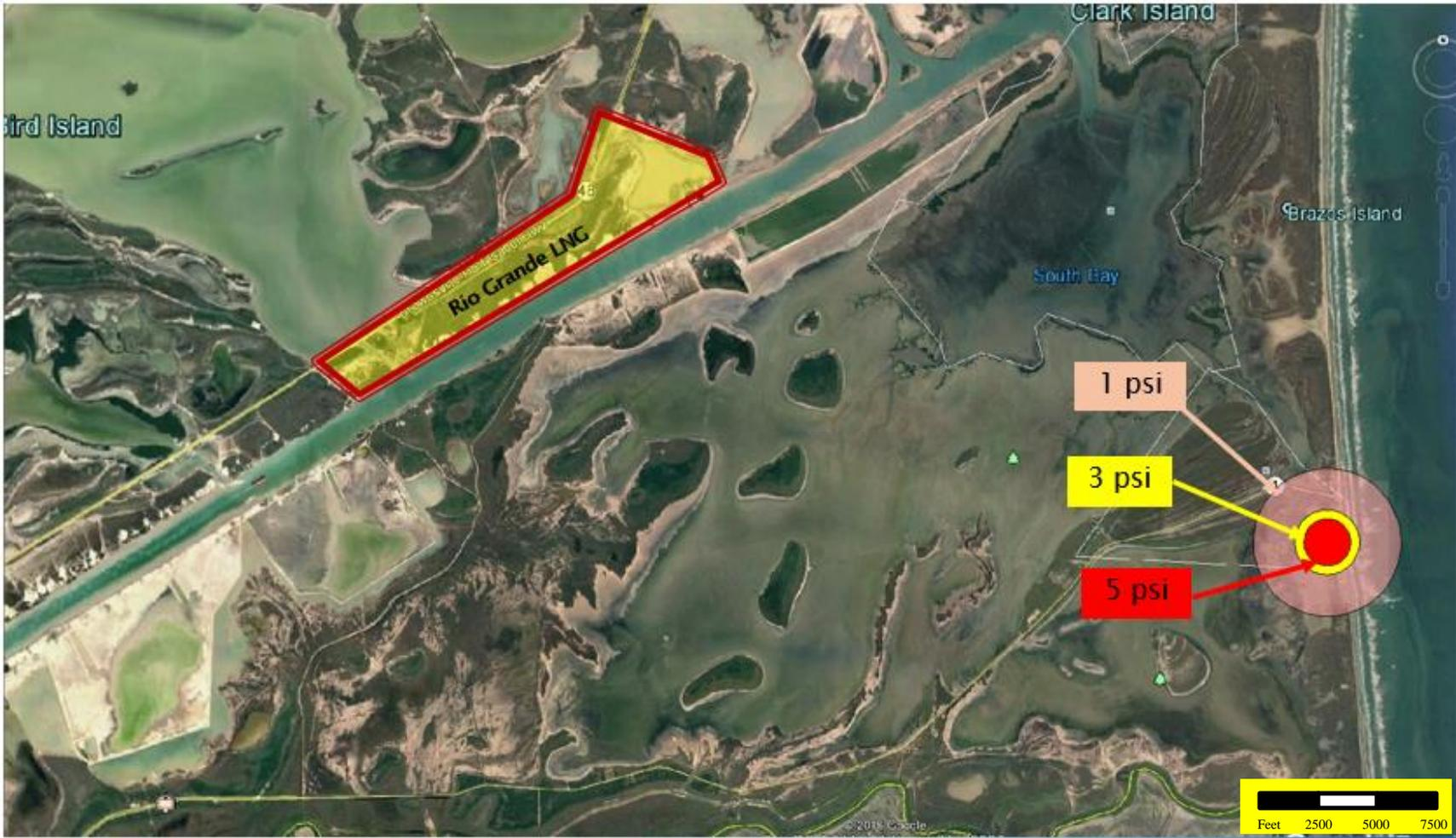
**Figure 8-1 Air Blast Overpressure Contours Resulting from a 322,200 Pound TNT Equivalent Explosion.**
