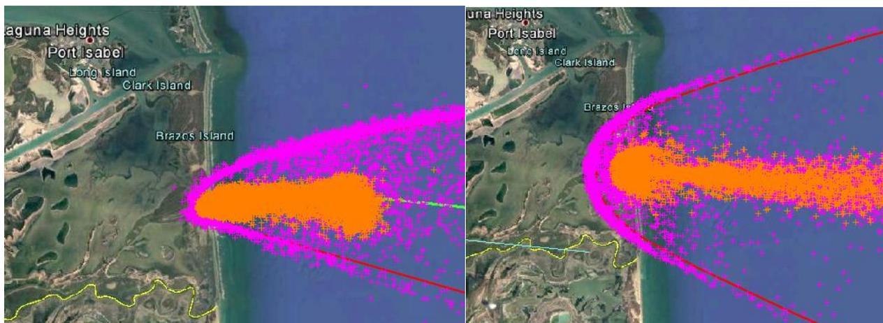
**Figure 6-1. Present Position of Vehicle at time of Thrust Termination (Orange + Marks) and IIP Points (Pink + Marks) for Falcon 9 V1.1 (left) and Falcon Heavy (right)**
