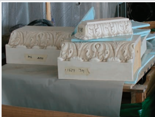
Detail of new terra cotta custom fabricated by Boston Valley Terra Cotta and installed by expert masons
