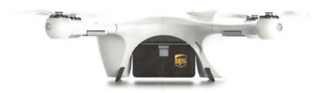
The M2 is typically flown from a ground control station (GCS) which utilizes a commercial-off-the-shelf device hosting a proprietary and secure aircraft control application. Communications with the sUA are accomplished via cellular signals. The M2 may also be controlled manually via a hand-held transmitter.
